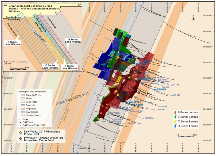
Figure 1: Plan map of the northeast plunging Gryphon mineralized lenses projected up to the simplified basement geology at the sub-Athabasca unconformity.
