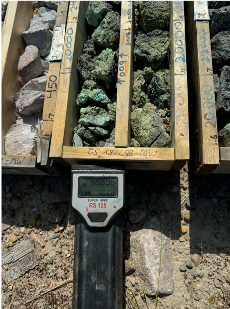
Figure 12-2: Confirmation of Mineralization via a RS 121 Scintillometer in MW-867
